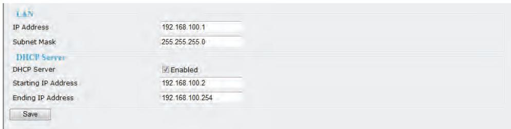
If you set up the network video recorder in LAN and link its LAN Port to network cameras and computer as the picture shows below, the DHCP server of network video recorder will automatically assign IP address to the linked devices. (192.168.100.2 ~ 192.168.100.254)
